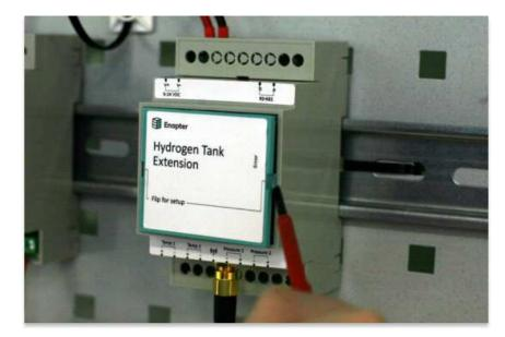
3. For factory reset press and hold "Reset" button and turn on power supply using breaker at the same time.
