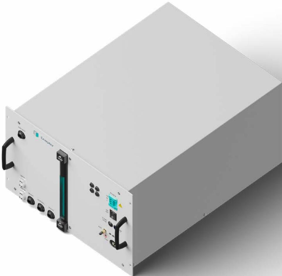
Enapter's Water Tank 4.1 provides storage for 28.5 litres of clean water for the AEM Electrolyzer. The water tank 4.1 is rack mountable into a standard 19" cabinet. The tank contains a conductivity sensor and a pump system to supply up to 12 AEM Electrolyzers with clean water.
